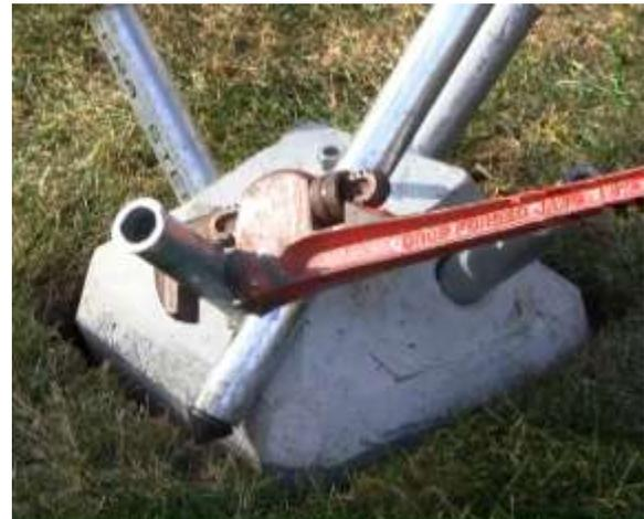
**Figure 6. Jacking Method for Pin Removal**
