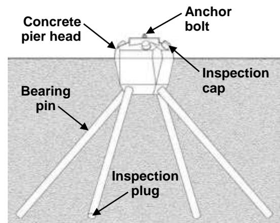
**Figure 1. Diamond Pier Foundation Components**
