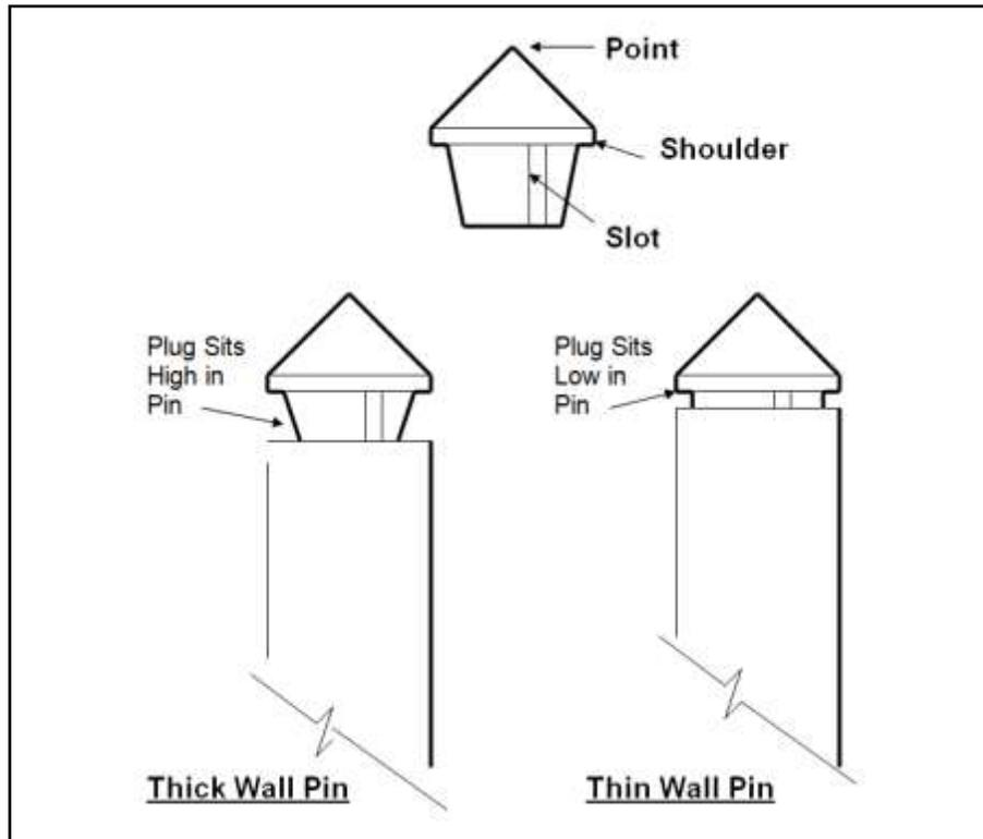
**Figure 8. Inspection Plugs**
